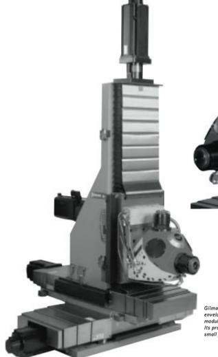
The installation of a turret head allowed the application of as many as six tools (HSK or ABS Mounting) to the work piece without physically removing and reinserting any tools.
