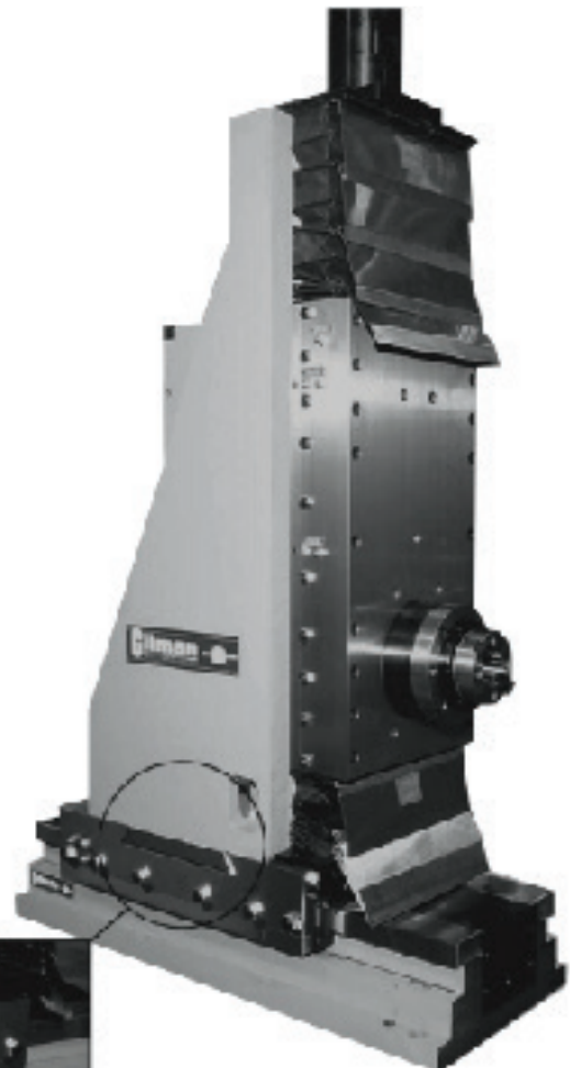
This Gilman Design feature allows 2" "X" axis adjustment without an additional slide.
