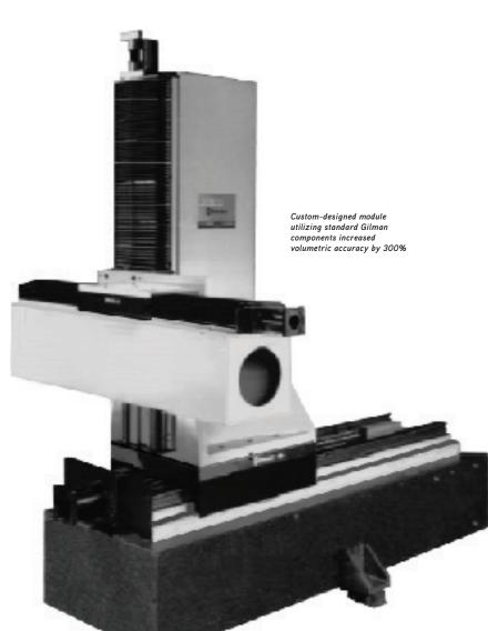
component was a key factor in the success of the project. IKO "Super X" series antifriction rollers were chosen by Gilman for their high vibration damping characteristics. The recirculating rollers of the "Super X" provide 2.6 times the rigidity of a ball-type guide-way of the same size, supplying accuracy needed for this application.
